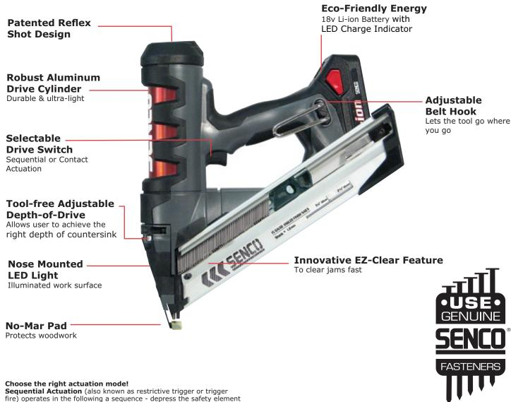
fire) operates in the following a sequence - depress the safety element at the nose of tool against the work surface then pull the trigger. After each fastener is driven, release the trigger and lift the tool off the work surface before starting the sequence again. This trigger is recommended and acceptable for most applications.
